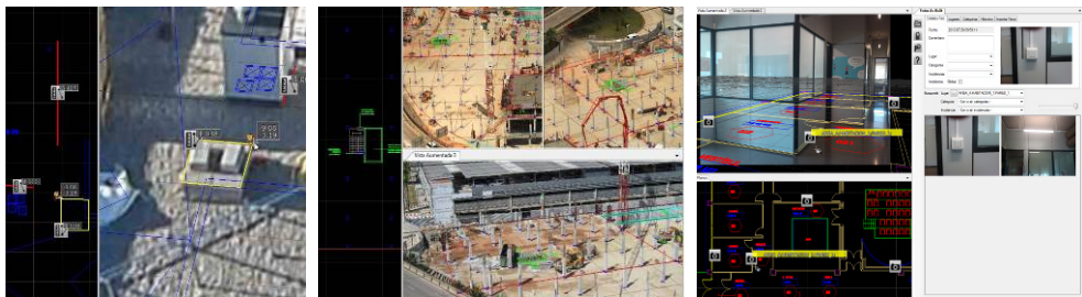
Fig. 9. Lineal and area measure (left); text and geometric annotations (center); as-built photo annotation (right).
