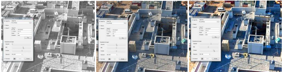
Fig. 6. Examples of the modification of brightness, contrast and saturation of the background images in the augmented views.
