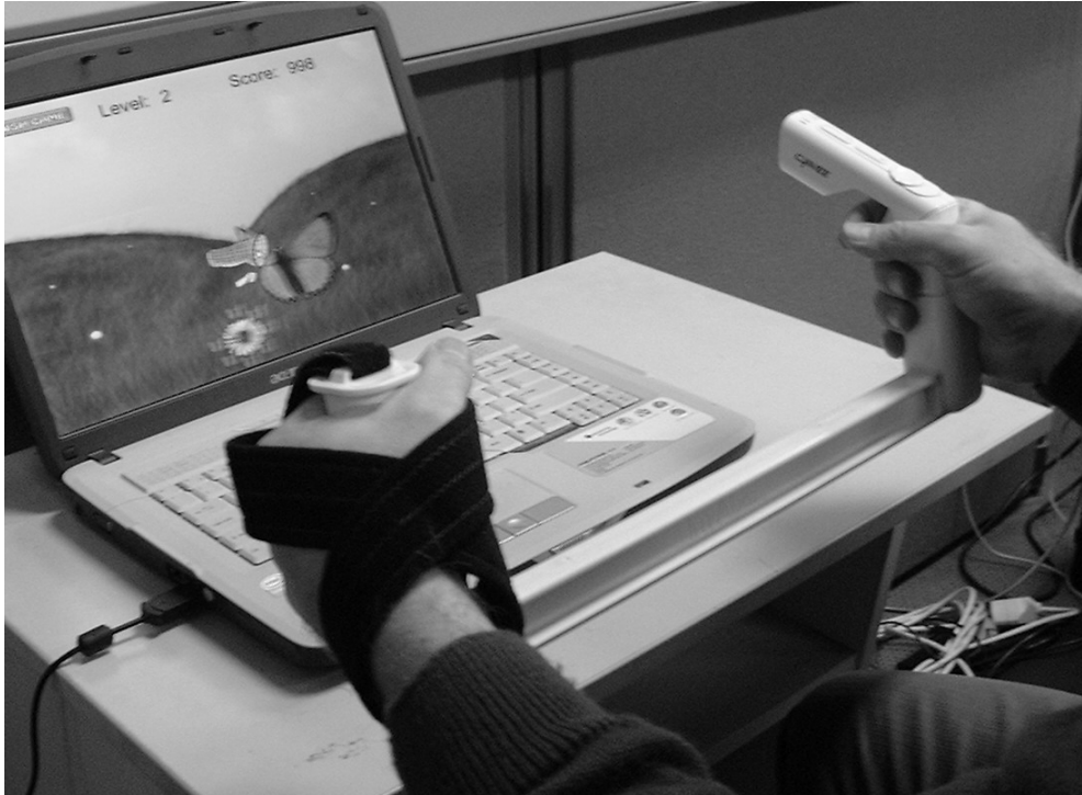
Fig. 2. Against-gravity bilateral exercise device that interacts with computer games.
