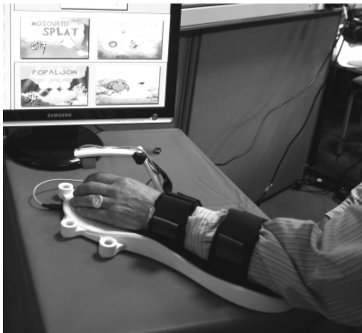
Fig. 7. Able-M, a gravity supported arm exercise device that interacts with computer games.
