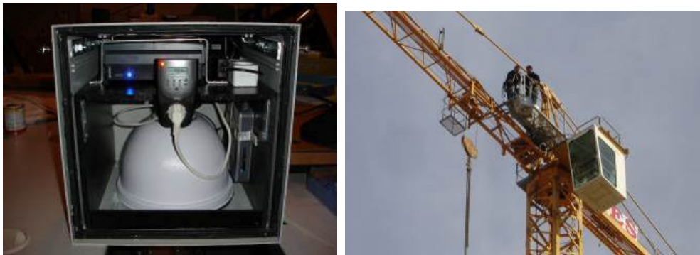
Fig. 3. PTZ camera (left); installation of the camera on a crane (right).
