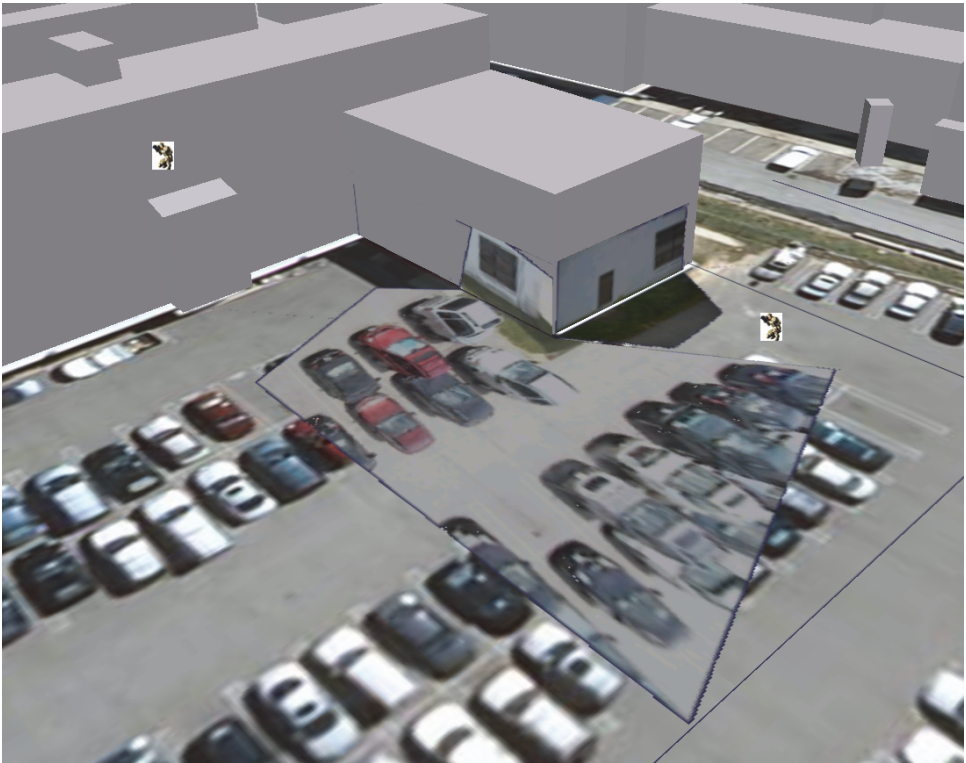
Fig. 4. Recreated 3D scene viewed with 3D buildings on Google Earth. The two field operator's icons and the video image are overlaid on Google Earth.
